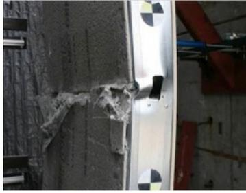
Figure 7: Hinge formed at utility hole.
