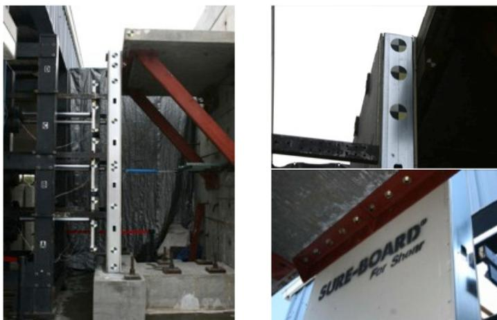
Figure 5: Test setup (left) and upper connection (right).
